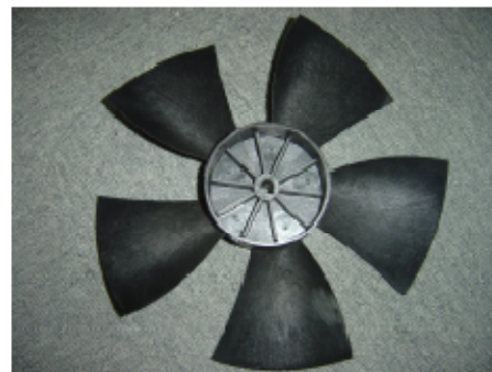
Fig. 1.1.2: Rotor, type SF01 – 300, material: AS with 20%GF
