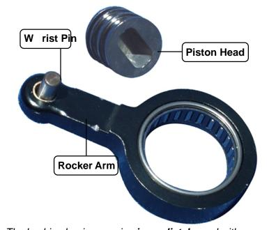
The bushing begins wearing **immediately**, and with continued use can wear out completely, leaving as much as a 0.063" gap. The result is a shorter piston stroke, **dramatically decreasing** recovery speed.
