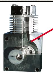
In other recovery machines, the crank-case is flooded with refrigerant to provide back pressure for the pistons. The constant presence of refrigerant subjects the internal components to the detrimental effects of corrosive materials.
