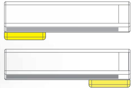
Gobi II pump can be mounted on the right or on the left side
