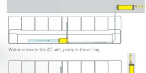
Water sensor inside the AC unit and pump outside the unit
