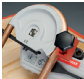
Forged aluminium segments with bending angle scale
