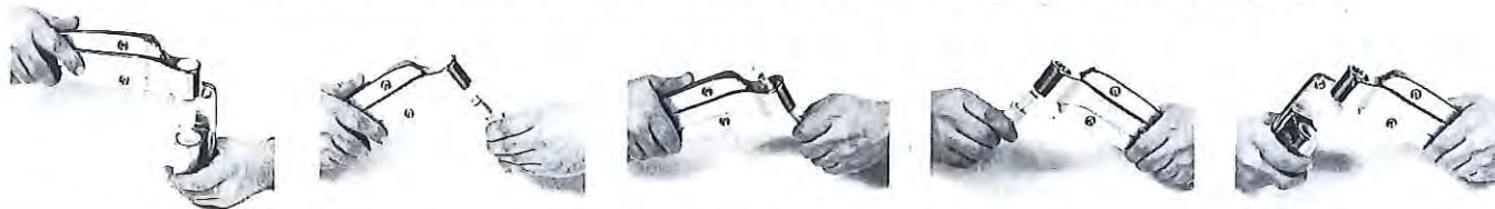
To reverse the 1245 lift strap from flange.
