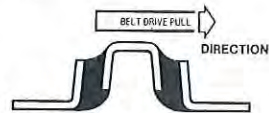
The M100 mountings provide excellent sideways stability with a good vertical isolation efficiency and are therefore ideal for belt drives, etc., but the mount should be installed with the tension as shown....
